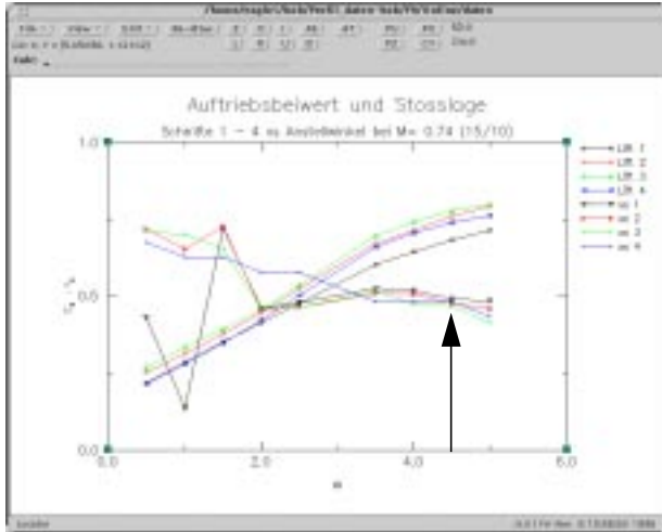
Figure 12: Lift coefficient and shock location vs. angle of attack, four wing sections. (Flow parameters equivalent to Figure 11)
