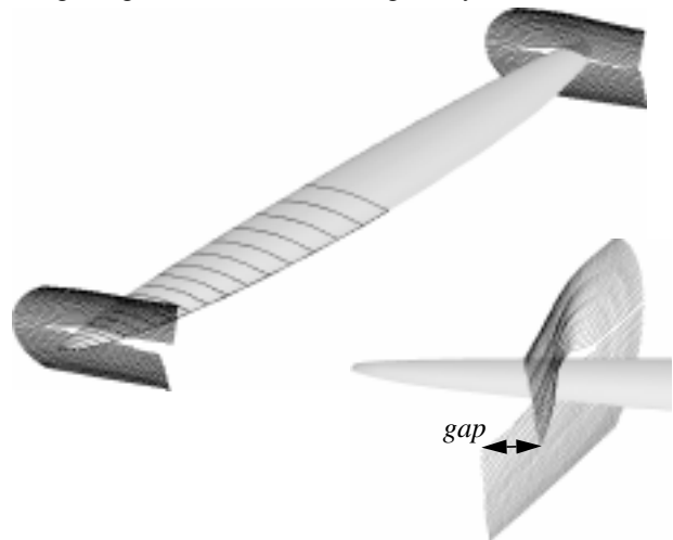
Figure 4: Stream surfaces past elliptic wing at 90% of halfspan, larger gap resulting from higher lift.
